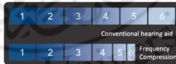
Figure 16. Illustration of frequency compression (from Starkey, with permission Crukley (2019)).
