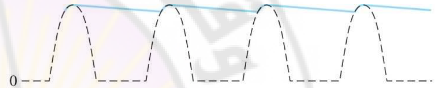
(b) Smaller ripple means more effective filtering. Generally, the larger the capacitor value, the smaller the ripple for the same input and load.
