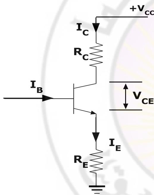
$$V_{CE} = V_{CC} - I_C (R_C + R_E)$$
