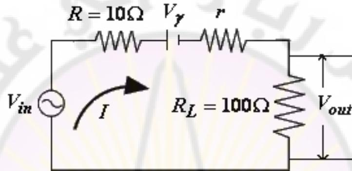
$$V_{in} = RI + V_{\gamma} + rI + R_L I$$
